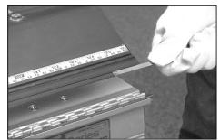
3 If installing full piece, start from either end of brake and slide ss strip into the grove until end is flush with extrusion. You may need to lightly tap the ss strip the last few inches.
