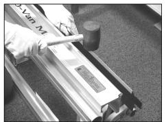
Turn brake over with castings facing down and extrusion is pointed up. Align the ss strip over the edge of the extrusion and tap on every few inches with a rubber mallet. Note: A block of wood, hammer and a helper can also be used. Be careful not to strike to hard so the block dents the ss strip.
