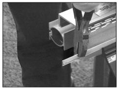
**2** Finish with pin punch as previously described. If ends appear to be loose, slide, or tap 2" of ss strip out past extrusion and pinch to tighten.
