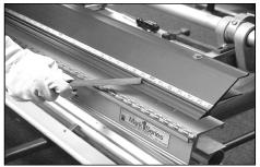
2 Clean groves in extrusion with mineral spirits or solvent. Remove visible burrs from extrusion that may interfere with ss strip using a fine file or sandpaper.
