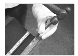
4 Pin punch the ends of the ss strip to prevent it from sliding off. Note: If the ss strip feels too hard to push, it may kink and damage. Stop and remove, go to Alternate install.
