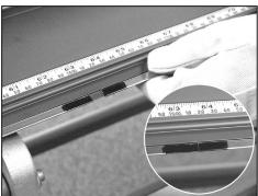
Locate the ends of the ss strip that have been painted black. These are the splice ends and should be in the center of the extrusion when done These ends have been over bent on the ends to ensure the splice will fit tight. Install using methods as described above.
