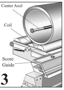
Note: As seen to the left, center coil with brake opening and allow material to pass freely through the brake without hitting castings.
