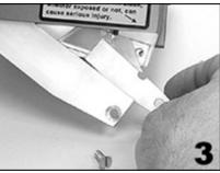
Carefully remove knife shim, set aside.
