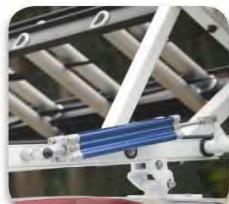
CONTROL LADDER DEPLOYMENT WITH ADJUSTABLE HYDRAULIC CYLINDER
