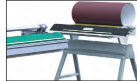
Coil Dispenser™ feeds materials into most brakes and slitters, preventing wind-blown damage and waste.
