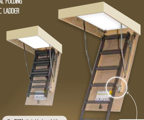
The **OWM** attic ladder has a folding metal ladder with a paintable noninsulated particle board hatch door. This model is mounted to the door with brackets that allow minor adjustments to the length of the ladder and the space between the ladder and door.
