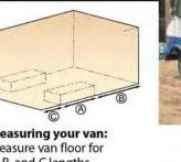
Measuring your van: Measure van floor for A, B, and Clengths as shown in drawing above. Compare shelving and/or module sizes to measurements of A, B, and C lengths. Overall sizes of shelving and modules are shown in charts on the following pages. When mounting shelving and/ or modules over wheelhouse (A), deduct two inches from shelving or module width for end panels. Installation should always be made to body frame member
