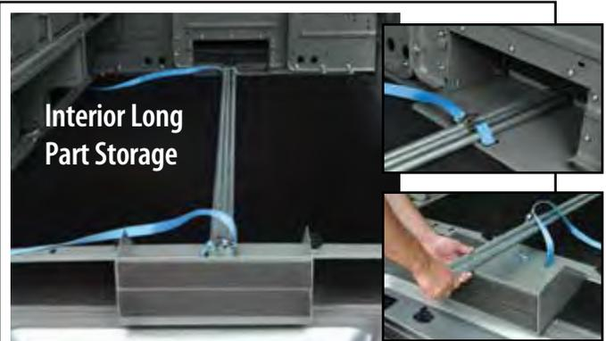
**Carry 10 feet of conduit or pipe inside your NV Cargo with the Long Part Storage Kit!**
