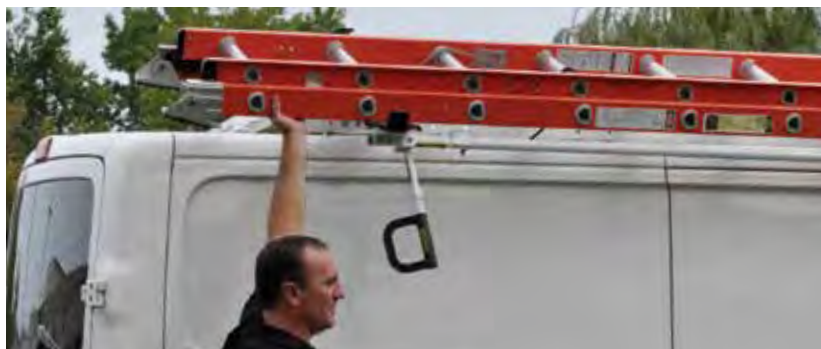
Lift ladder off the rear bracket.
