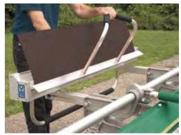
Unimount™ (included) allows use of Unilegs™ No. UNL1, or can be added to the back of any "Mark" series brakes.
