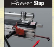
Allows Q-Cutter to remain installed on the track without interfering with bending. Simply slide Q-Cutter back to stop. Quick release allows for easy removal for transport.
